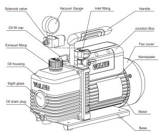
Remark: Only new refrigerant series are assembled with solenoid valve and vacuum gauge
